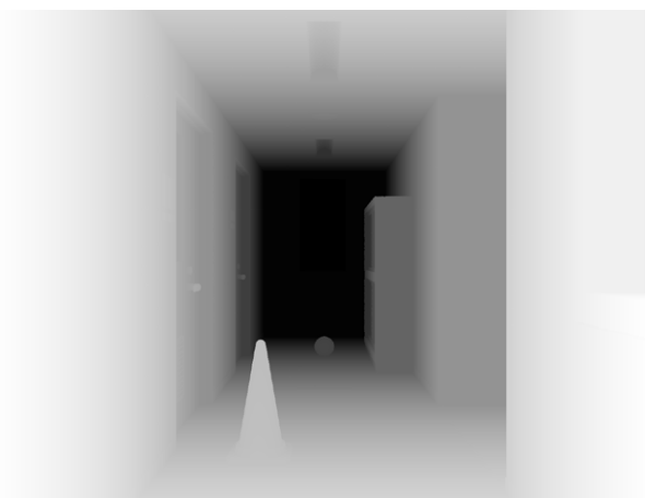
Fig.6 Depth map of the CG image. This image represents the distance map of the objects in Fig.5.
